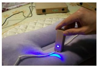
F.8 The simple Tester is merely for testing if the materials or accessories are suitable to conduct anion.
